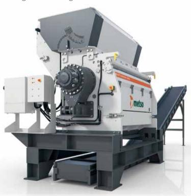
The multi-edged shaft is fitted with a patented knife system and is fed by a pusher. The sensitivity of the pusher ensures that material is not forced onto the shaft and a minimum of heat is generated. The hydraulic drive of the shaft guarantees impact resistant and
